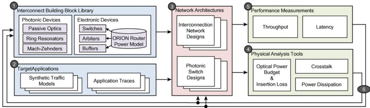
Fig. 1. Design flow of modeling a network in the PhoenixSim environment.
