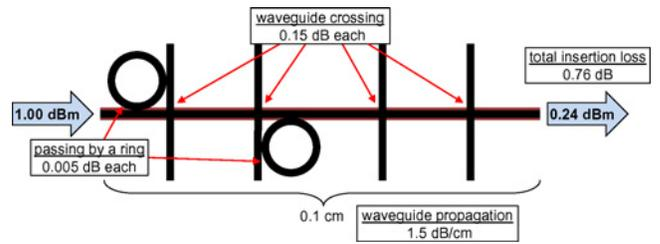
Fig. 9. Calculation of insertion loss for a small network segment.
