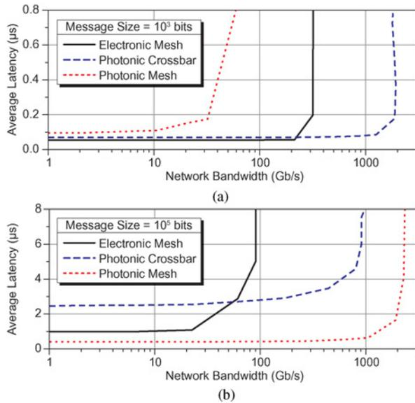
Fig. 15. Bandwidth and latency performance on the Electronic Mesh, Photonic Crossbar, and Photonic Mesh for (a) 1-kbit and (b) 100-kbit message sizes.
