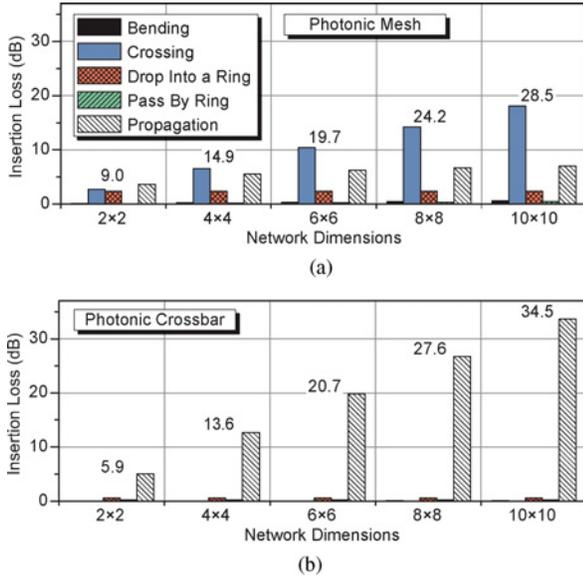
Fig. 13. Insertion loss results for the (a) Photonic Mesh and (b) Photonic Crossbar of varying sizes. Labeled values that overlay the columns indicate the worst-case total network-level loss values. Columns illustrate the worst-case loss associated with the individually labeled loss component which does not necessarily occur in the network path with the worst total loss.
