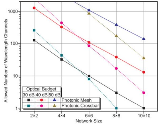
Fig. 14. Wavelength channel allotment in the Photonic Mesh and Photonic Crossbar for varying network sizes and optical power budgets.
