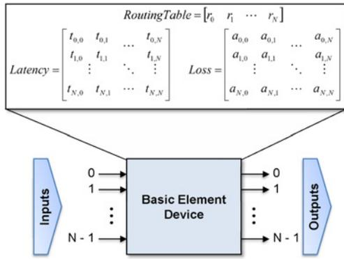
Fig. 4. Parameters for characterizing a photonic device using the *Basic Element Model*.
