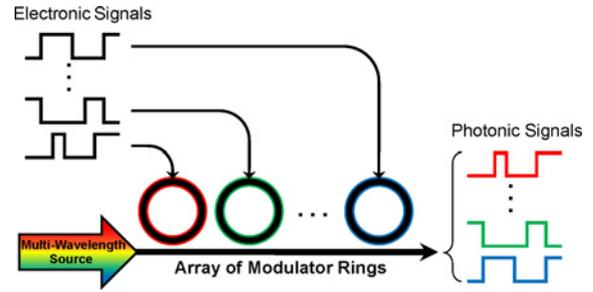
Fig. 7. Schematic of the conversion process between the spatially parallel electronic domain and wavelength-parallel optical domain.
