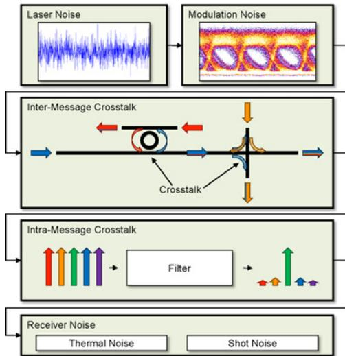
Fig. 10. Sources of noise and crosstalk within a chip-scale photonic system.
