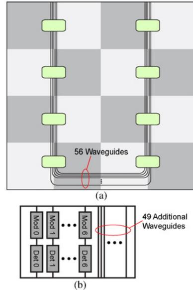
Fig. 12. Photonic Crossbar topology. (a) High-level representation of a  $2 \times 4$  Photonic Crossbar, connecting 16 cores. Boxes represent gateways with a concentration of two processing cores. (b) Detail schematic of the Photonic Crossbar gateway, showing 49 bypass waveguides and seven waveguides with modulator and receiver banks used to communicate to the other seven gateways.
