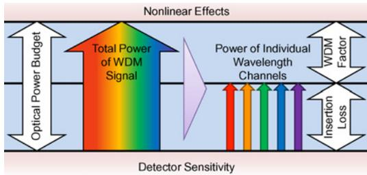
Fig. 8. Relationship of various parameters affecting the optical power budget. The difference in power of the total WDM signal (large arrow on the left) and the individual wavelength channels (five smaller arrows on the right) constrains the scalability of the system.
