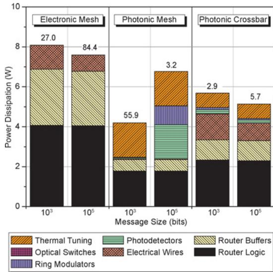
Fig. 17. Network-level power dissipation breakdown of the Electronic Mesh, Photonic Mesh, and Photonic Crossbar for transmission of 1-kbit and 100-kbit messages. Values overlaying each column indicate the energy efficiency of the network in units of pJ/bit.
