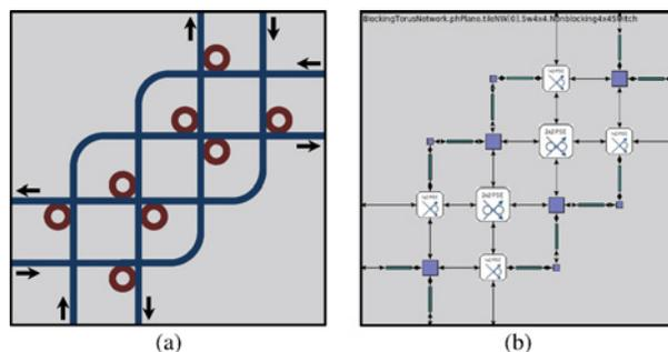
Fig. 3. (a) Schematic of a design for a  $4 \times 4$  nonblocking photonic switch. (b) Screenshot of how PhoenixSim composes the switch by instantiating basic photonic devices.
