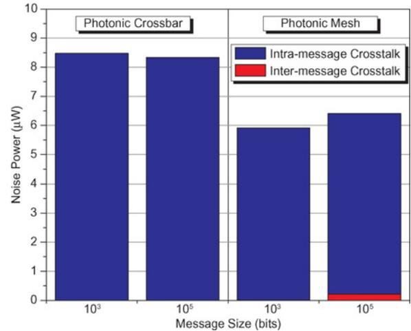
Fig. 16. Average total noise power accumulated by each optical message in the Photonic Mesh and Photonic Crossbar for saturated network load. Laser noise, thermal noise, and shot noises are negligible quantities and are not listed.
