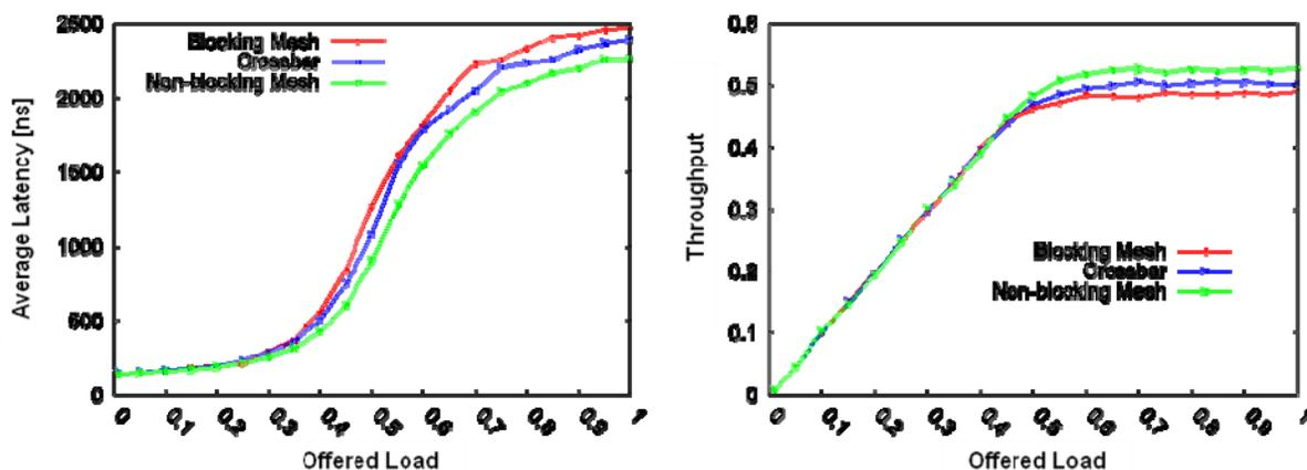
Fig. 4: Simulated latency and throughput performance evaluation for various 36-port network architectures.
