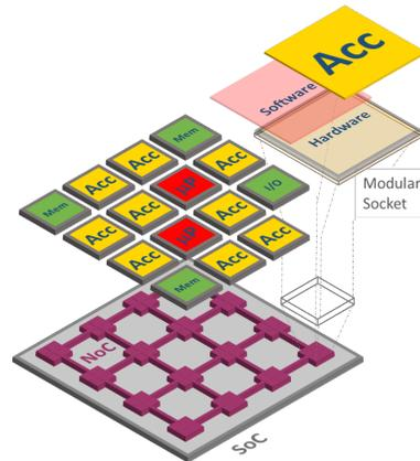
**Figure 1: Integrating heterogeneous components in an Embedded Scalable Platform.**
