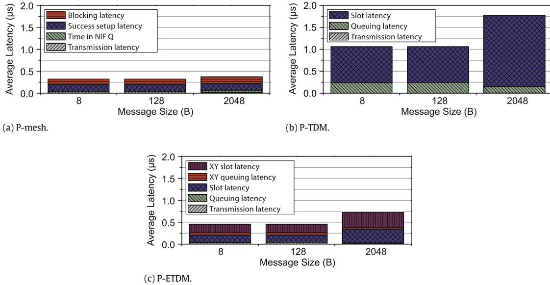
Fig. 11. Half-load latency breakdown under Uniform traffic.
