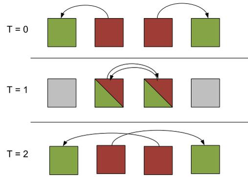
Fig. 2. Row communication TDM slot examples for four nodes. (For interpretation of the references to colour in this figure legend, the reader is referred to the web version of this article.)
