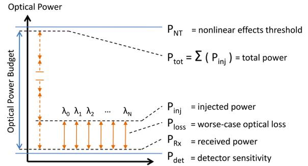
**Fig. 8.** Number of wavelengths dictated by insertion loss and optical power budget.
