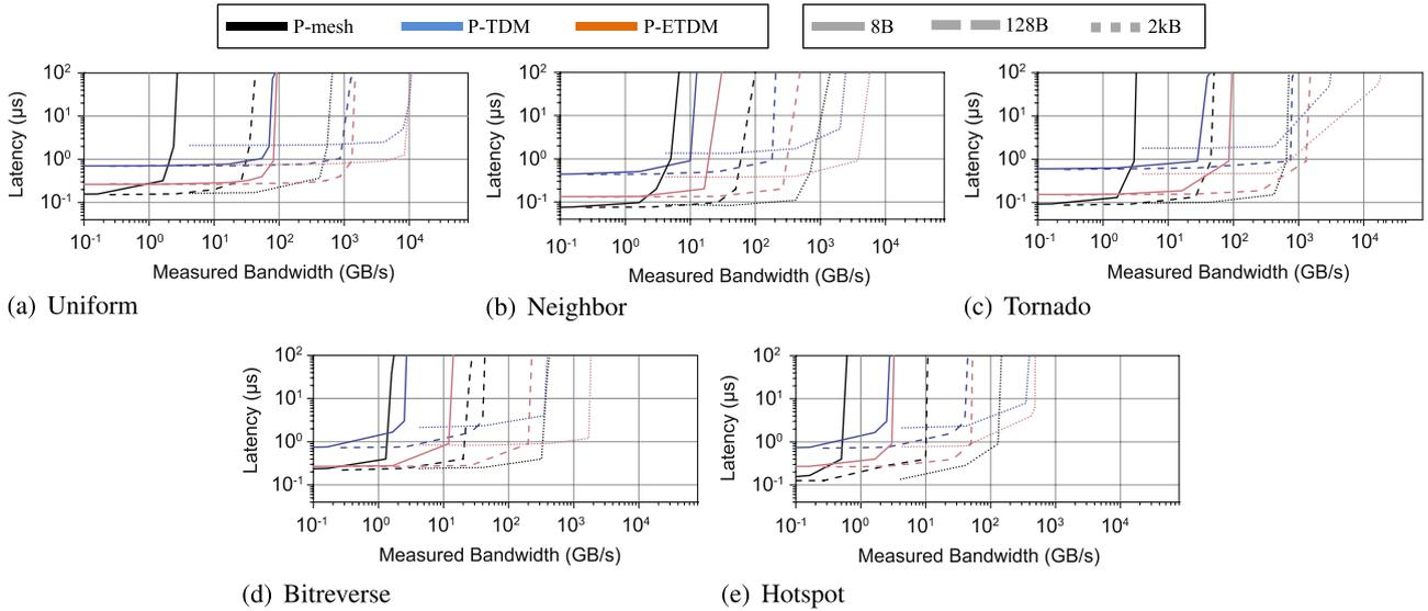
Fig. 9. Latency vs. bandwidth under synthetic traffic.
