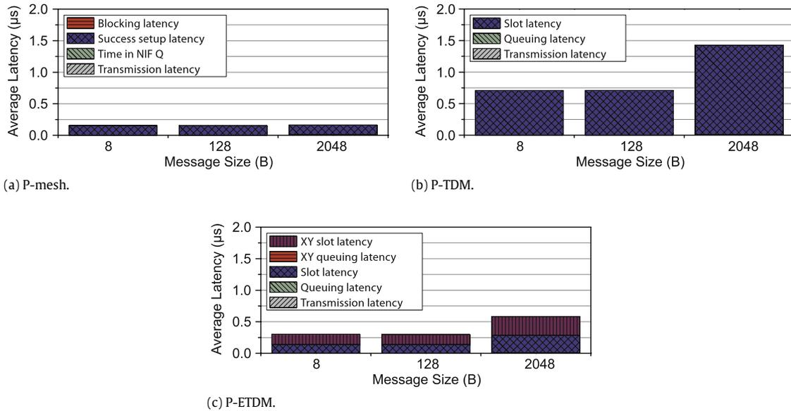
Fig. 10. Zero-load latency breakdown under Uniform traffic.
