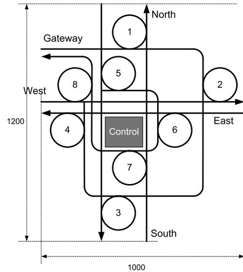
Fig. 5. Layout of photonic switch, showing waveguides and ring resonators. Units in microns.
