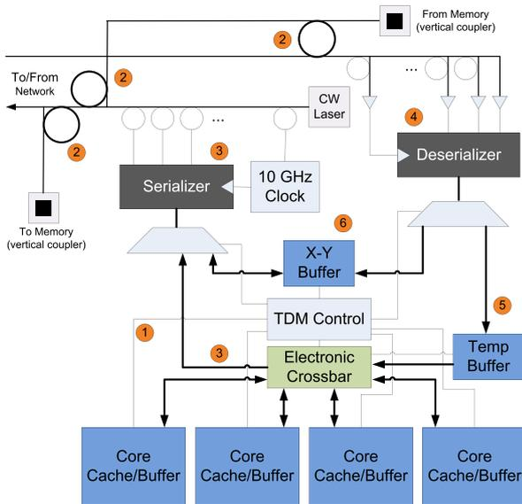
Fig. 6. Network gateway microarchitecture.
