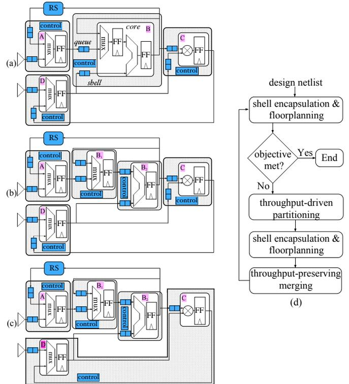
Fig. 1. (a) A simple LI system with four cores and one RS; its throughput is  $2/3 = 0.67$ . (b) The same system with a finer-grained shell encapsulation where core  $B$  is split in two smaller cores  $B_1$  and  $B_2$ ; throughput is improved to  $3/4 = 0.75$ . (c) The LI system maintains the same throughput after core  $C$  and  $D$  are merged. (d) The proposed high-level physical synthesis flow.
