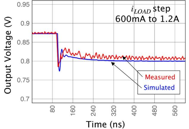
Fig. 10. Measured and simulated load-current transient step response.
