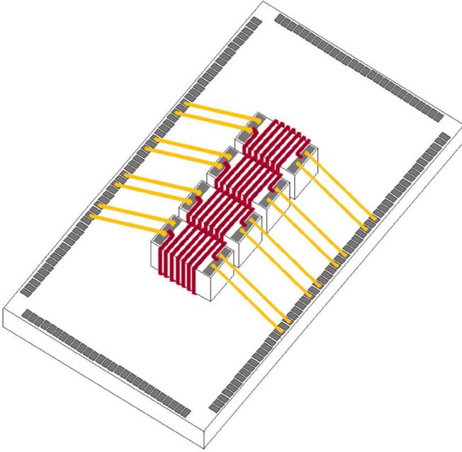
Fig. 9. Illustration of SMT inductor integration by bondwire connections.
