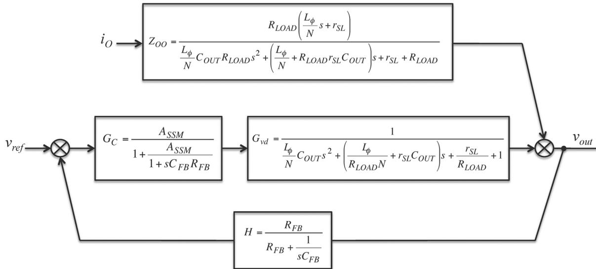
Fig. 6. Small-signal model of control loop.
