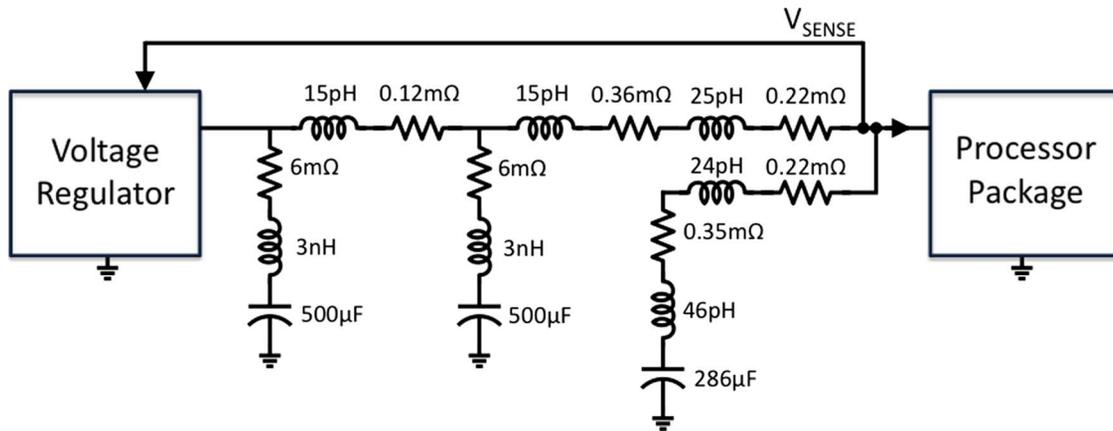
Fig. 1. Power Distribution Network for a modern high-performance microprocessor, from VRM to CPU package [5].
