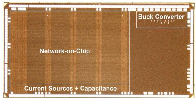
Fig. 8. Photo of test chip.
