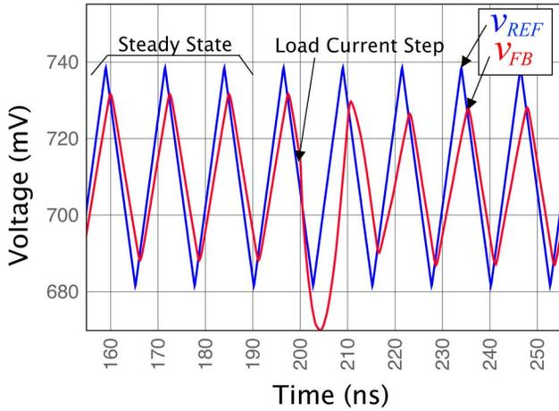
Fig. 4. Simulation of  $v_{REF}$  and  $v_{FB}$  during steady state and load transient.
