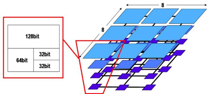
Fig. 14. Network-on-chip architecture.
