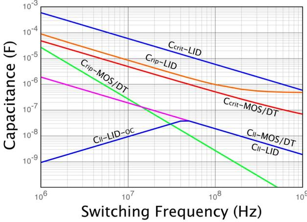
Fig. 2. The minimum capacitance meeting constraints for an IVR with operating parameters defined in Table I. Voltage ripple ( $C_{rip}$ ), load-line regulation ( $C_{II}$ ) and the saturating transient response ( $C_{crit}$ ) are plotted versus converter switching frequency,  $f_{sw}$ , for low-inductance discrete capacitance (LID) and on-chip MOS or DT capacitance.
