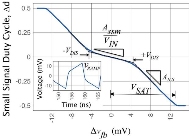
Fig. 5. Small signal change in duty cycle,  $\Delta d$ , as a function of small signal deviation from steady state  $v_{fb}$  with  $D = 0.5$ . Inset: effective PWM ramp  $v_{ramp}$ .
