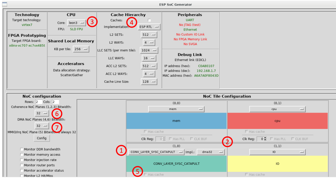
Figure 5: The ESP GUI, labeled with options students can change during their SoC-level DSE.
