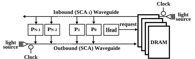
Fig. 6. The P-sync Architecture
