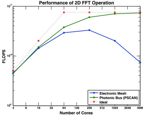
Fig. 13. Simulated performance in floating-point operations per second of the electronic mesh architecture (blue) and P-sync architecture using PSCAN (green) for 2D FFT. Ideal performance shown by red curve.
