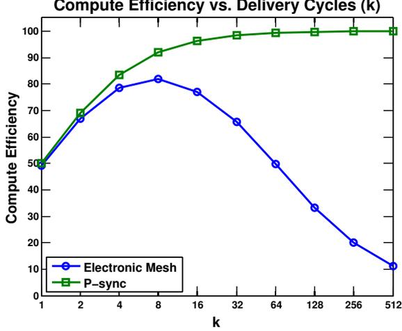
Fig. 11. Global synchrony and pre-scheduled communication allow P-sync to achieve near ideal FFT compute efficiency as  $k$  increases. Such efficiency gains in the mesh are limited by the increased overhead of routing smaller packets.
