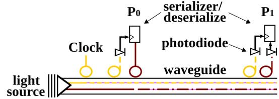
Fig. 3. Transmission and reception of a photonic message (red) between two processors  $P_0$  and  $P_n$  synchronized by a global photonic clock (yellow).
