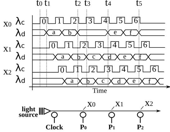
Fig. 4. SCA operation: Each processor location  $P_0$ – $P_2$  contains a detector and modulator. The timing diagram represents the clock and data wavelengths,  $\lambda_c$  and  $\lambda_d$  respectively, traveling past the waveguide locations  $x_0$ – $x_2$ .
