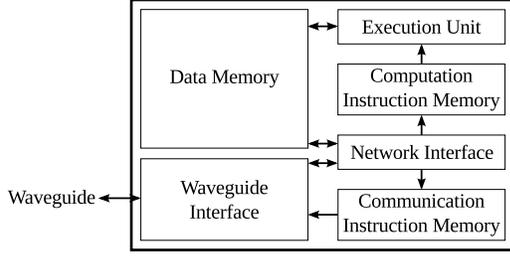
Fig. 7. The processor architecture of a P-sync node enables the SCA and  $SCA^{-1}$  communication modes.
