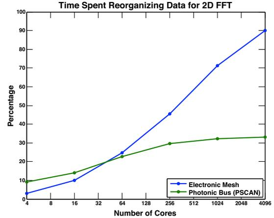
Fig. 14. Percentage of runtime spent in reorganizing data for the 2D FFT on the electronic mesh (blue) and P-sync (green) architectures.
