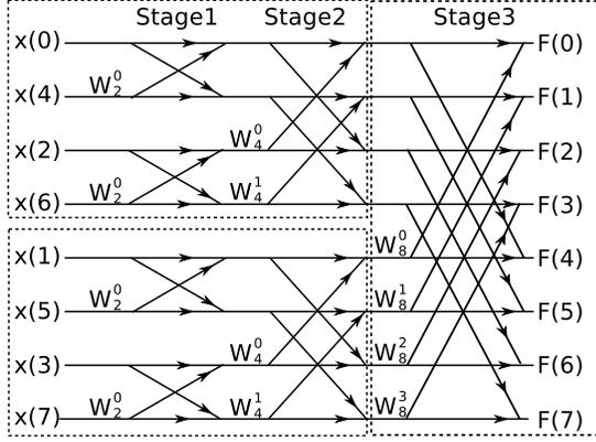
Fig. 10. The FFT can be broken down into smaller, more local computations. Dotted lines are shown for  $k = 2$  delivery cycles, each four elements in size.
