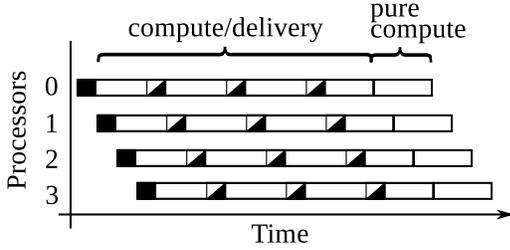
Fig. 9. Model II: Blocked data delivery model.
