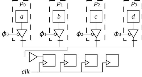
Fig. 1. Electronic time domain multiplexing bus with four processors,  $P_0$ – $P_3$ , clocked by  $\phi_0$ – $\phi_3$  and containing data bits  $a$ – $d$ , respectively. Processor outputs feed an electronic shift register with  $clk$  frequency locked to  $\phi_i$ .
