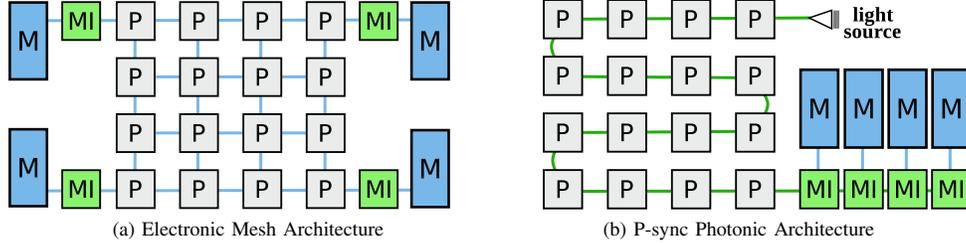
Fig. 12. Both architectures contain processing (P), memory (M) and memory interface (MI) elements.
