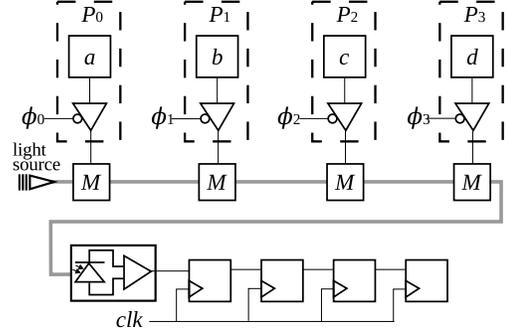
Fig. 2. Photonic time domain multiplexing bus in which each processor  $P_i$  has a modulator  $M$  sending data to the shift register via a photodiode receiver circuit.
