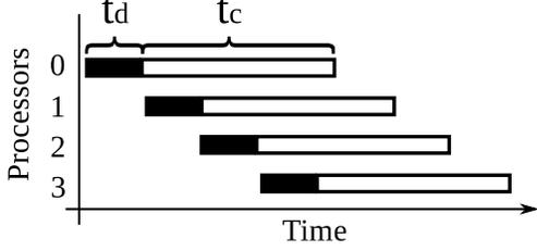
Fig. 8. Model I: Simple data delivery model.
